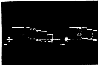
① VIDEO INPUT SIGNAL (50mV/10ms) Pin ③① of IC301 (PAL Color bar input: 1.0Vp-p)
